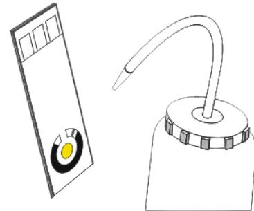
**B** Or put electrode of SPE into DI water or buffer solution of you prepared at 5~10 min.
